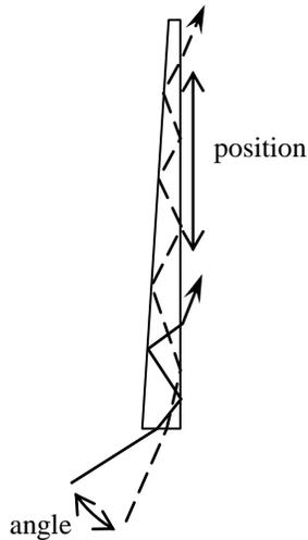
Fig. 2: In a wedge, input angle determines a ray's end position.
