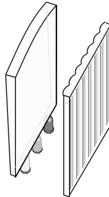
Fig. 31: The guide collimates light from each LED and the lenslets concentrate light through the appropriate color filter.
