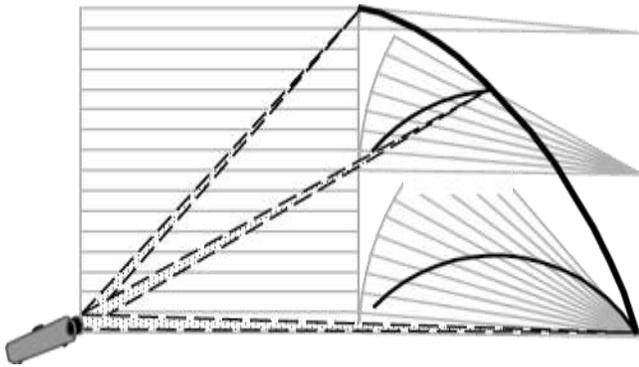
Fig. 13: Optical path length through a slab plus wedge varies little with ray input angle
