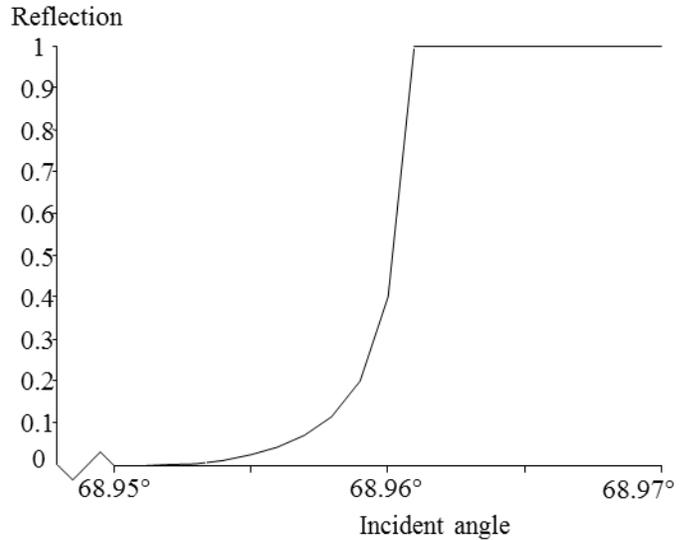
Fig. 11: Predicted fraction of polarized monochromatic light reflected at a dielectric interface with a two layer coating
