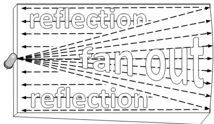
Fig. 27: rays fan out and reflect off the thick end which is curved so as to collimate them.
