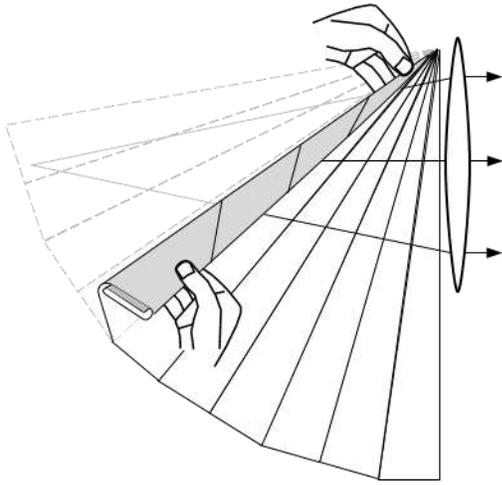
Fig. 5: The light-guide folds up the space between lens and focal plane
