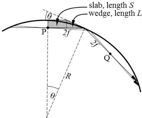
Fig. 17: The kink between slab and wedge smooths into a curve (thick line) which collimates rays from a point at the input
