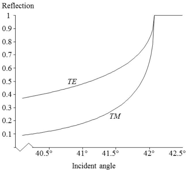
Fig. 10: Predicted fraction of incident light reflected at an uncoated acrylic air interface
