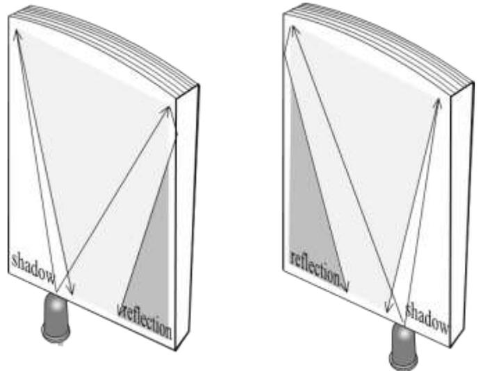
Fig. 36: The shadow left by one LED can be filled by its equidistant opposite from the centerline
