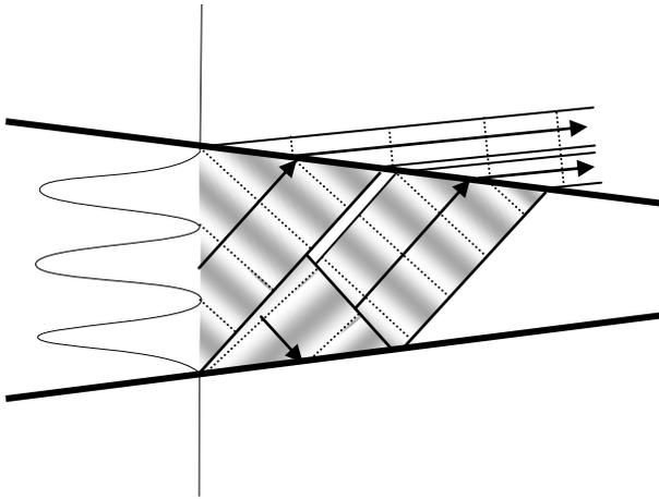
Fig. 9: The mode emerges like a pair of counter-propagating rays
