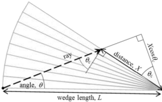
Fig. 6: A ray inside a wedge travels like a straight ray through a stack of wedges
