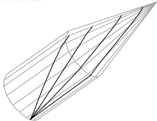
Fig. 16: The path of rays through a slab then wedge can be unfolded onto a curved surface
