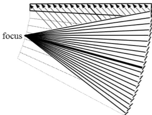
Figure 29: Emboss the thick end with facets to reduce ray angle and guide rays to focus
