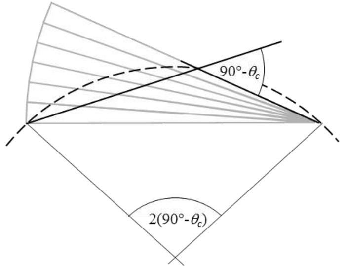
Fig. 7: By the inscribed angle theorem, projection via a thin wedge is like projection inside a cylinder
