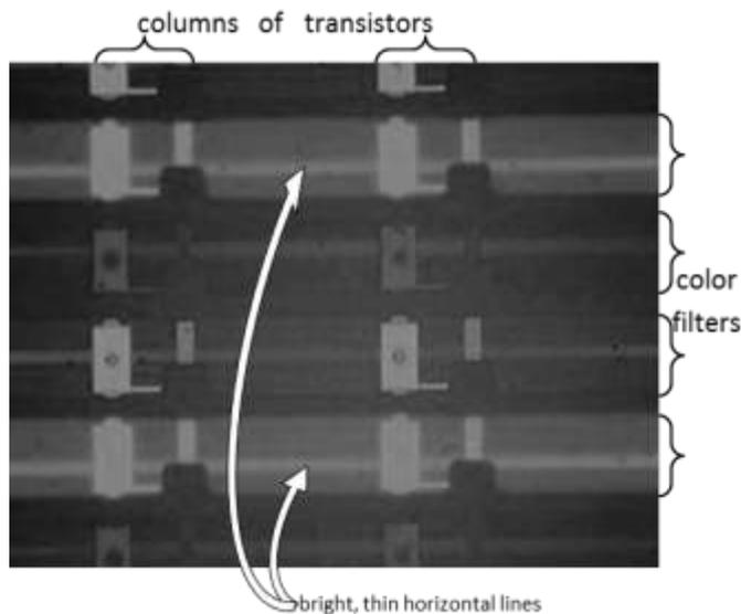
Fig. 32: Photograph showing light (the bright, thin horizontal lines) being concentrated through the center of each color filter.
