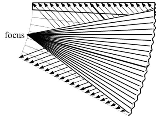
Fig. 30: By symmetry, the facets must be a zig-zag so rays exit from top and bottom
