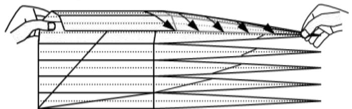
Fig. 15: The path of rays through a slab then wedge cannot be unfolded onto a flat plane without breaks
