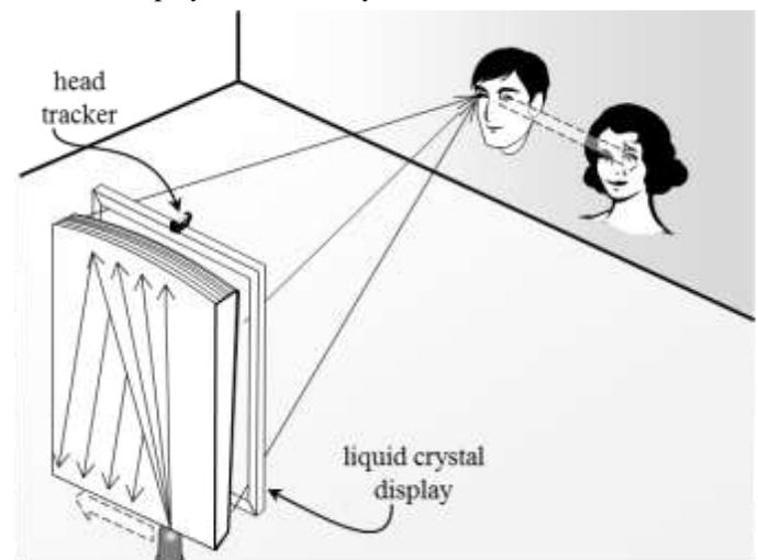
Fig. 33: Rays through the liquid crystal display are concentrated to each eye in turn found by the head tracker
