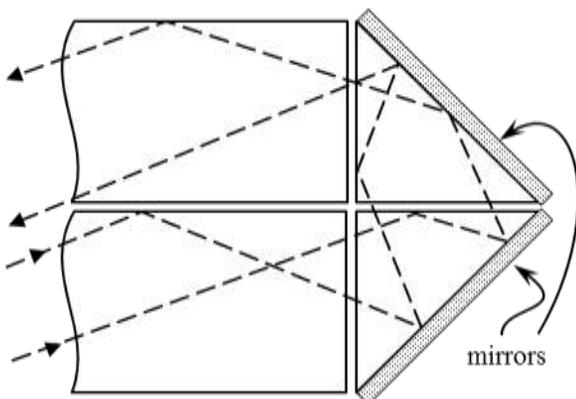
Fig. 18: A pair of prisms can fold a light-guide but not easily
