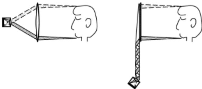
Fig. 21 Imaging through a wedge light guide is like imaging through a lens.
