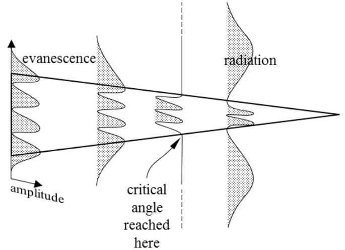
Fig. 8: The peaks of a mode converge like a spring until the critical angle is reached
