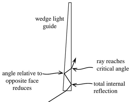
Fig. 1: Each reflection off one face of the wedge reduces the ray's angle to the other face
