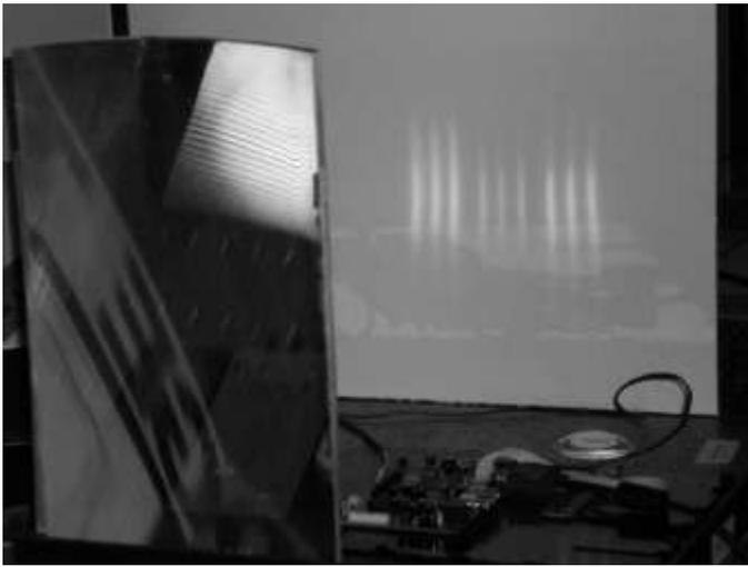
Fig. 34: Photograph of the image formed on a screen in front of a wedge backlight with a Fresnel lens against its exit surface and nine LEDs at its thin end.
