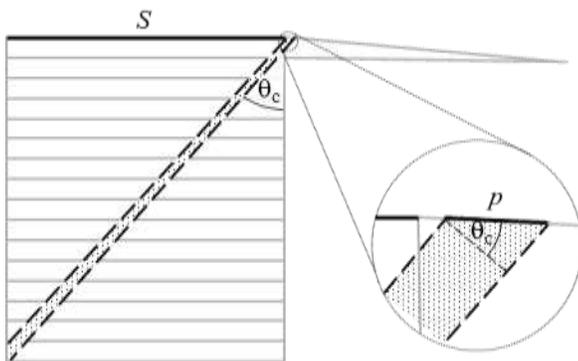
Fig. 14: A pixel can be smaller than the light-guide thickness if a ray bundle is convergent.
