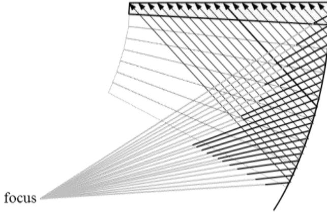
Fig. 28: We want all rays to exit at the critical angle. Trace them backwards and reflect off the thick ends
