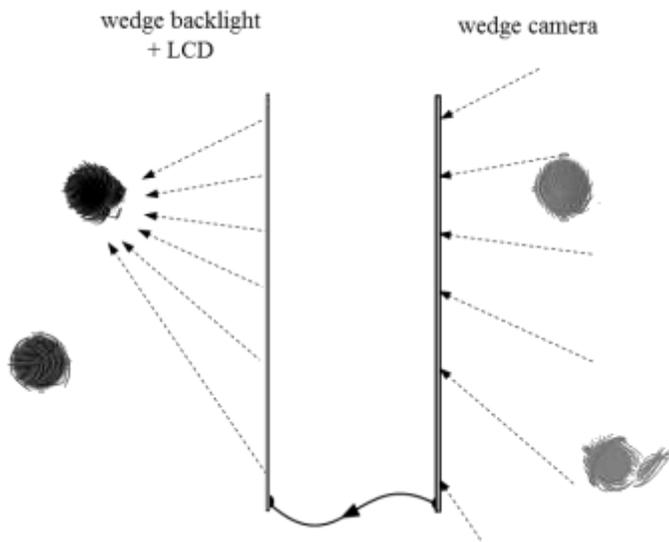
Fig. 35: A wedge camera and wedge backlight have the potential to televise the experience of looking through a window
