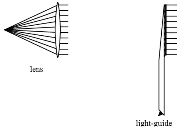
Fig. 4: Rays leave a wedge at the critical angle so all are collimated, as with a lens
