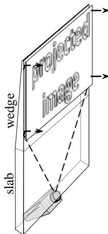
Fig. 3: Insert a slab so rays can fan out to the width of the screen
